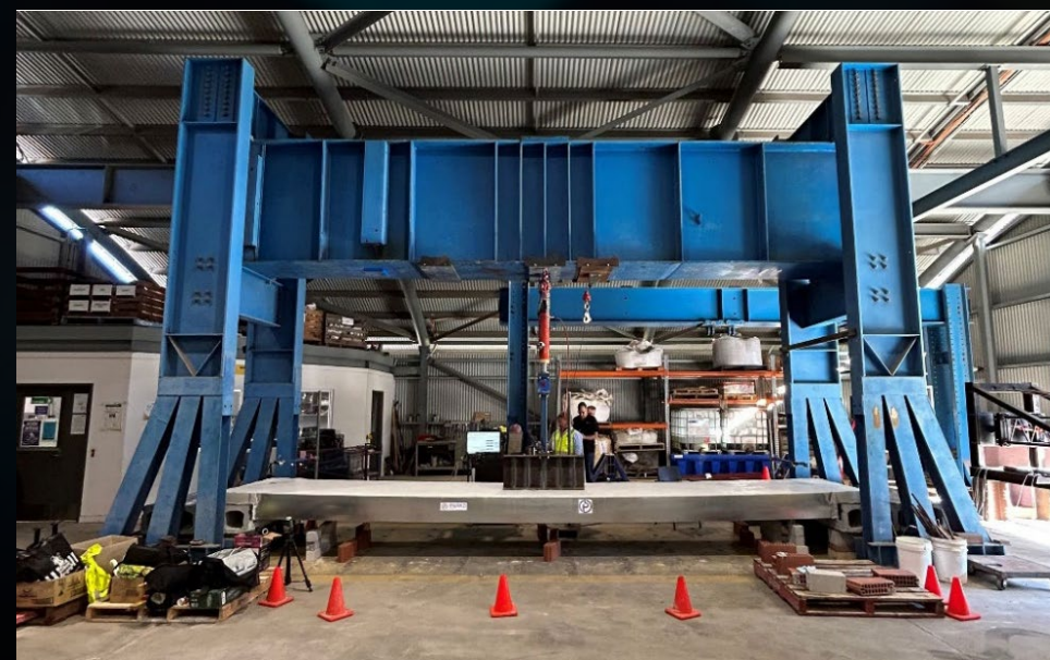
Load Test for PARKD system in Perth, WA
